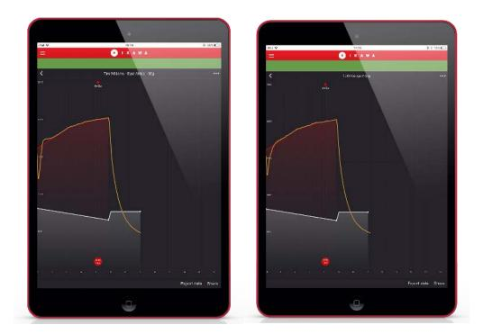
We have added a new, predictive element within the temperature control algorithm which allows the roaster to react immediately to changes in fan speed or temperature, and has also helped minimise overshoot in the early stage of the roast.
